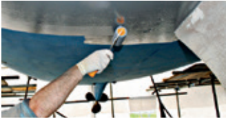
Apply Hempel's High Protect with roller
