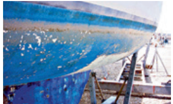
Paint blisters and lifts
